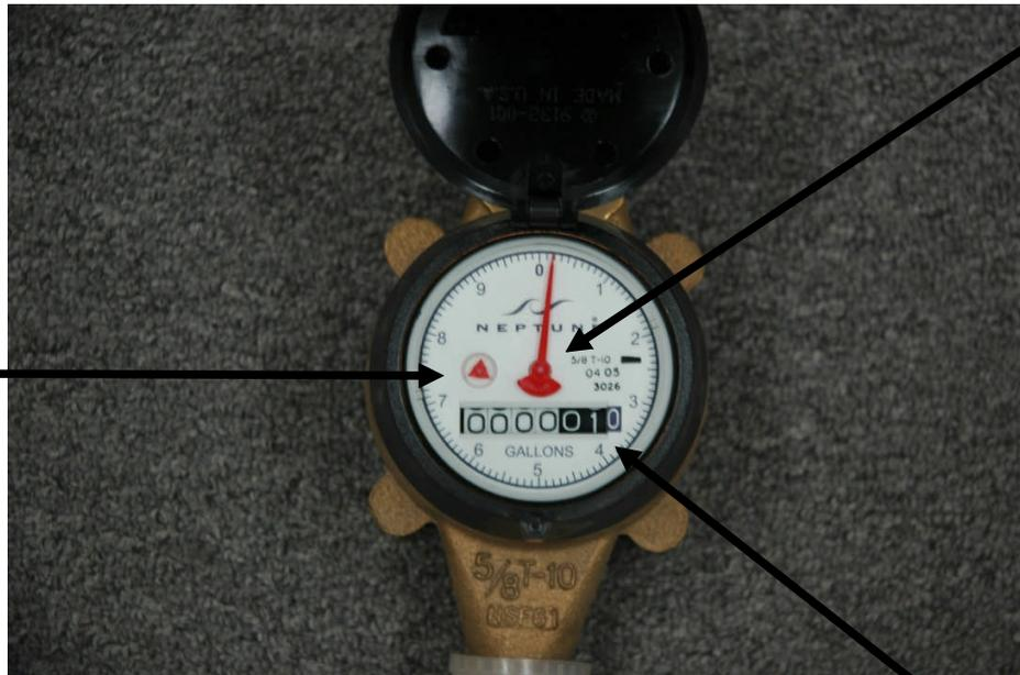
This is the actual reading. The meter has a fixed zero, measuring in tens of gallons. For every revolution of the sweep hand, the digit next to the fixed zero will register. If you check this before you water and again immediately after, you will have a good idea of how much water you are using in your yard.
